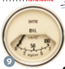
Oil temperature gauge mechanical fitting (racers fit to sump plug location using HPS8 union. P68 No.23)
