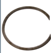
Clip for holding outer track of nose bearing in clutch case. 2A3643
